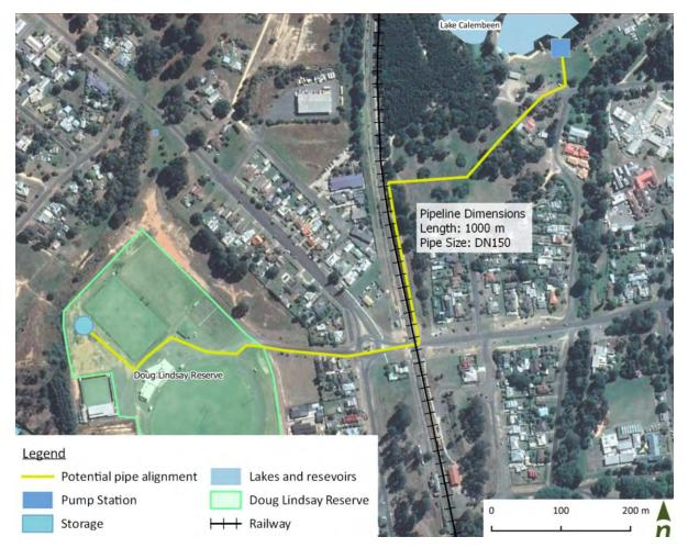
Figure 6. Raw water from Lake Calembeen infrastructure requirements
