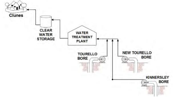
Figure 20. Clunes potable water system schematic (Source: Central Highlands Water)
