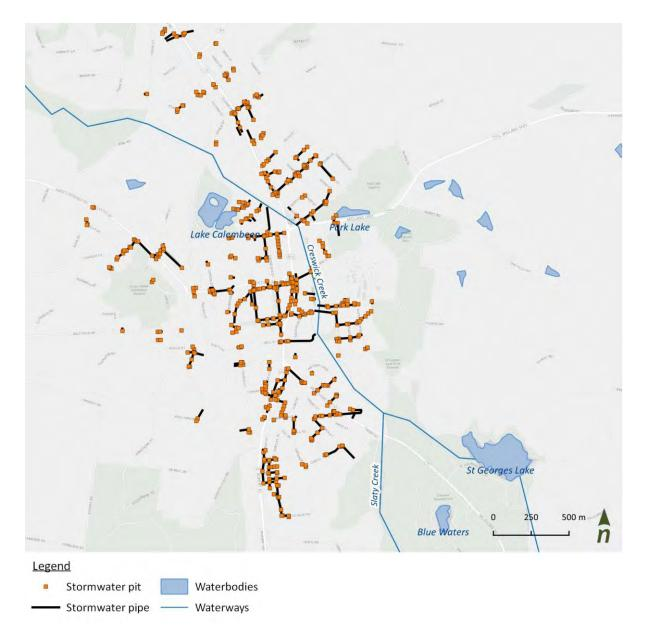
Figure 27. Stormwater drainage network in Creswick (Data: Hepburn Shire Council)
