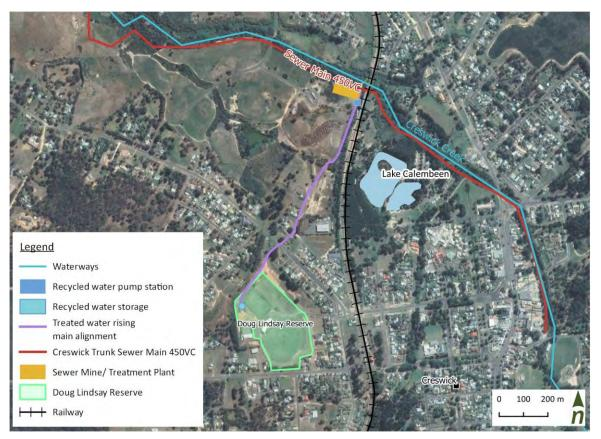
Figure 12. Proposed sewer mining arrangement
