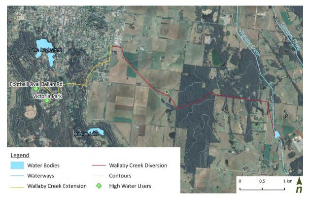
Figure 9. Proposed arrangement of transfer network from Wallaby Creek Diversion to Victoria Park
