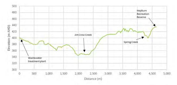
Figure 7. Elevation profile of pipeline alignment from the Shepherds Flat WWTP (at distance zero) to the Hepburn Reserve
