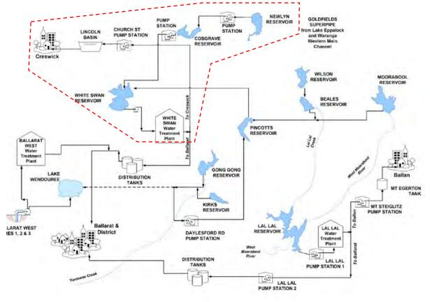
**Figure 17** Ballarat potable water system schematic – Creswick system outlined in red-dashed border (Source: Central Highlands Water)
