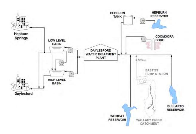
Figure 15. Daylesford potable water system schematic (Source: Central Highlands Water)
