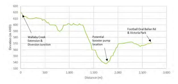
Figure 10. Elevation profile of pipeline alignment
