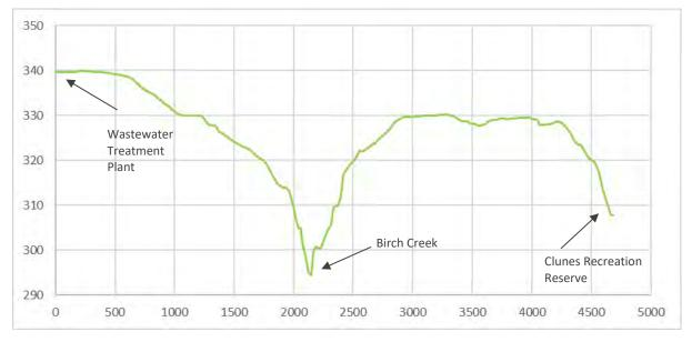
Figure 5. Elevation profile of pipeline alignment
