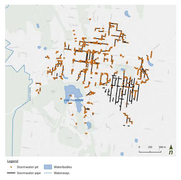
Figure 26. Stormwater drainage network in Daylesford (Data: Hepburn Shire Council)
