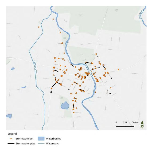
Figure 28. Stormwater drainage network in Clunes (Data: Hepburn Shire Council)
