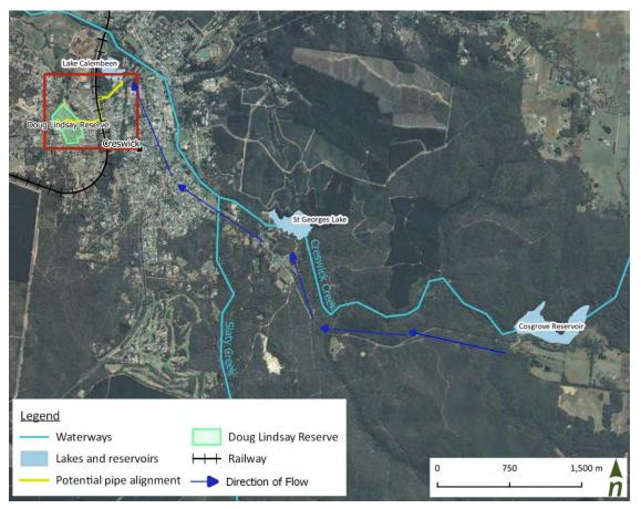
Figure 5. Raw water from Lake Calembeen arrangement overview (inset in Figure 6 below)
